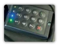
Standard Pin Panel Access, you can manually enter the password, also supports RFID card swiping to start. This function greatly simplifies the process of authorized operation, especially when multiple personnel can operate the vehicle.
