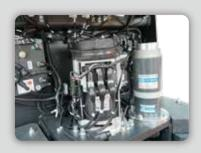
Powerful AC drive: AC drive motor designed and manufactured by Schabmueller, KORDEL gearbox, vehicle speed up to 5mph. In addition, Rader Vogel or Wicke drive wheels imported from Germany extends the service life of the PU.
