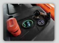
The multi-function instrument can display the vehicle working status, battery power, working time, driving speed and steering angle. The outer ring aperture of the instrument will change from green to red, and the fault code will be displayed when maintenance is required.
