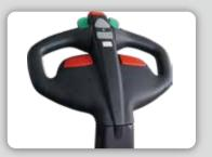
German REMA handle with reliable and ergonomic control system. In addition, the non-contact lifting and lowering rocker switch extends the life of the handle.
