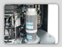
The standard electric power steering system used in Noblelift stackers can quickly and accurately control the position of the steering wheel, while meeting the standards, with high reliability and safety.
