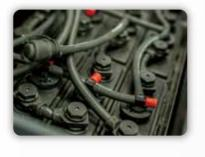
The vehicle can be equipped with an automatic filling system to quickly refill the lead-acid battery.
