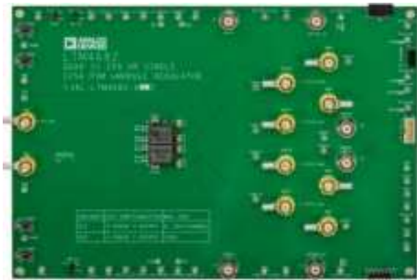
Figure 1. EVAL-LTM4682-A1Z Evaluation Board (Part Marking is either ink Mark or Laser Mark)
