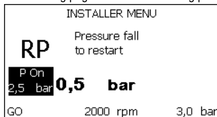
Figure 18.1: Setting the restart pressure (2)
