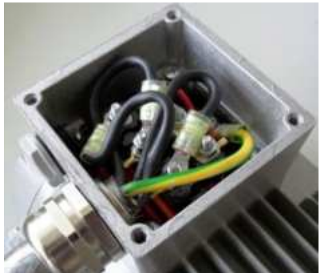
Fig. 25: Wiring on the motor connection box
