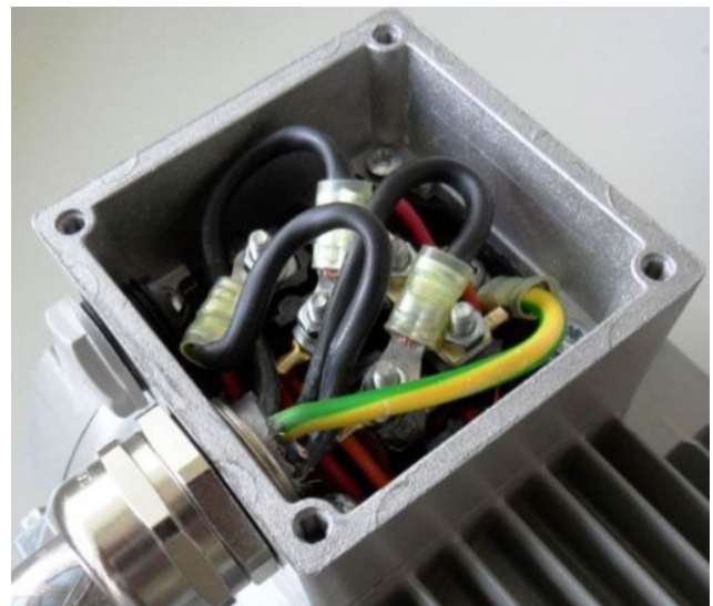
Fig. 32: Wiring on the motor connection box
