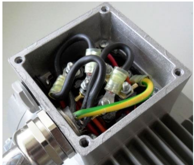
Fig. 25: Wiring on the motor connection box
