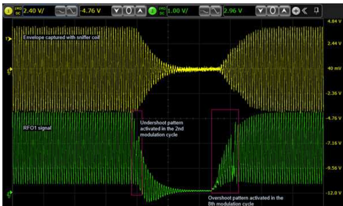
Figure 12. NFC-A waveform with overshoot and undershoot pattern activated
