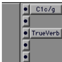
A TDM insert point with TrueVerb after the +C1.
