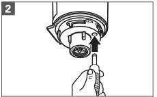
Plug in the Charger Adapter Pin into the Charging Port.
