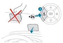
Press and hold button 2 to deactivate the system and retract the blade.
