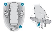
To unlock the loading area alone, the remote control on your person in recognition zone A, B or C, pass your hand behind a handle of the front left or right doors, then pull the handle to open the corresponding door. Depending on the version, the door mirrors unfold only when the cabin is unlocked, the alarm is deactivated.
