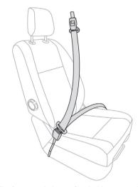
The front seat belts are fitted with a pyrotechnic pretensioning and force limiting system.
