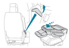
Pull the control fully up and tip the backrest forward.
