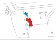
Before refitting the seat in the vehicle, pull the strap fully to ensure that the latching mechanism has engaged.
