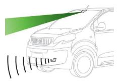
The vehicle has a camera located at the top of the windscreen and a radar located in the front bumper.
