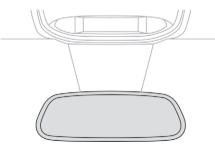
This system automatically and progressively changes between day and night use by means of a sensor measuring the light coming from the rear of the vehicle.
