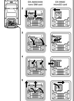
NOTICE Even when not using a microSD or nano SIM card, be sure to close and lock the slot cover(s).
