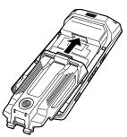
2 Attach the unit to the main unit by using two fingers to push the two parts of the unit indicated with arrows until they click.
