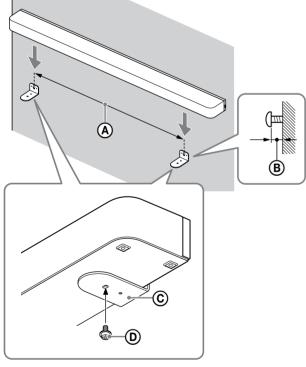
(a) Distance between the screws (commercially available) for wall installation: 876 mm (B) Gap between the wall installation screw head and wall: 3.5 mm to 4.5 mm
