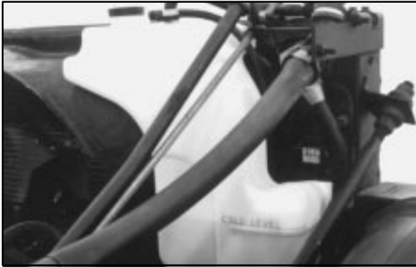
Coolant Recovery Tank (Gasoline Engines -- Sloped Hood)
