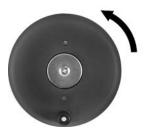
Drive shaft (valve) turns counterclockwise in direction OPEN.
