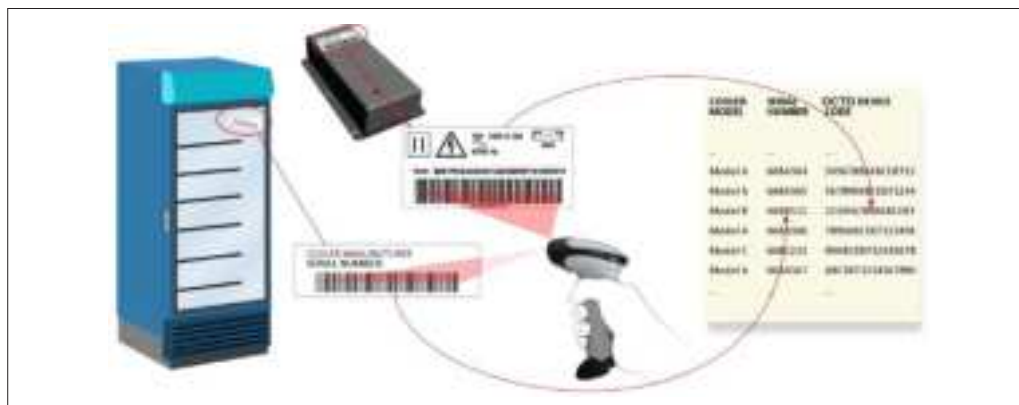
Fig. 8: Association between OCTO device and the specific cooler.
