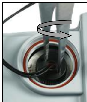
Use a tweezer to unscrew the lamp cover.
