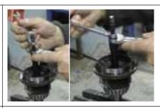
Use two wrenches to expand the chuck to roughly clamp the bearing inner hole.
