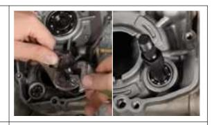
2. Use two wrenches to expand the chuck to roughly clamp the bearing inner hole.(Wrench is not included in this product)
