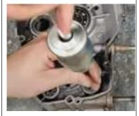
3. Screw the hammer into the clamp connection thread. (Select part: P)
