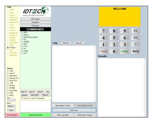
The Universal SDK Demo app displays VP3350's available commands in a command tree, as shown above. Single-click on a command to populate the center panel of the window with optional settings relevant to the command (for example, "Amount" and "Start EMV Additional Tags" above). In some cases, text fields appear, allowing users to enter custom values.
