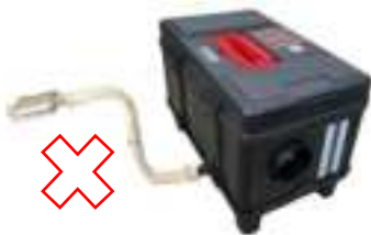
Incorrect Installation Direction
