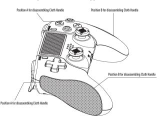
When the fabric surface is dirty, the fabric support can be disassembled and cleaned with water, it can be easily disassembled from the position A or the position B indicated in the above figure. After the fabric surface is cleaned and dried, buckle on the fabric support and the main body.
