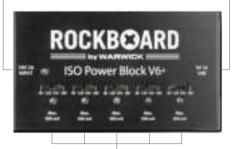
5 x switchable slots with 9V DC / 12V DC / 15V DC / 18V DC; Individual maximum output: 500 mA at 9V, 375 mA at 12V, 300 mA at 15V, 250 mA at 18V
