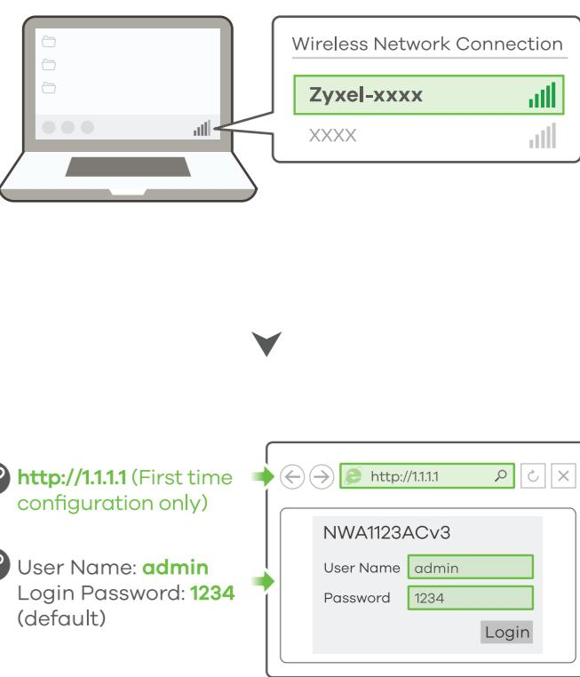
EN ① From a WiFi enabled computer, search for the NWA1123ACv3's default WiFi network name (**Zyxel-xxxx**, where xxxx is the last four characters of the MAC address) and connect to it.
