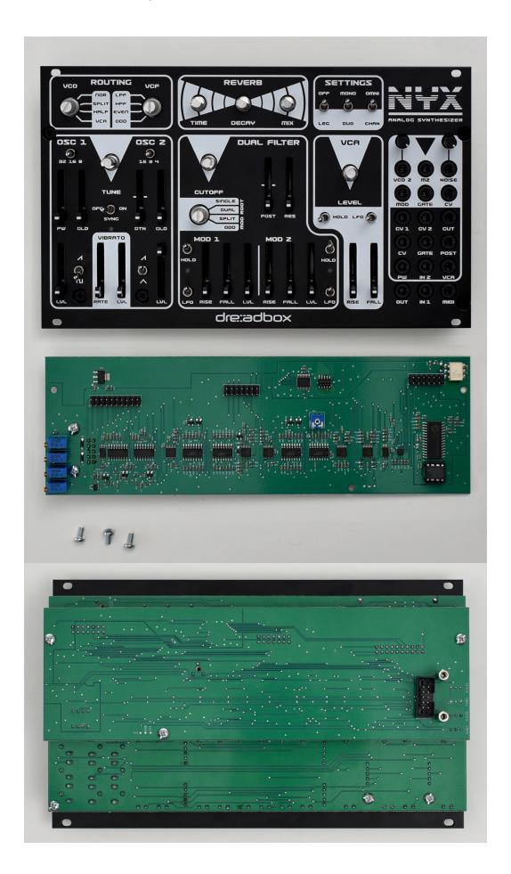
Attach the power board to the assembly as shown and secure with 2xM3 brass screws.
