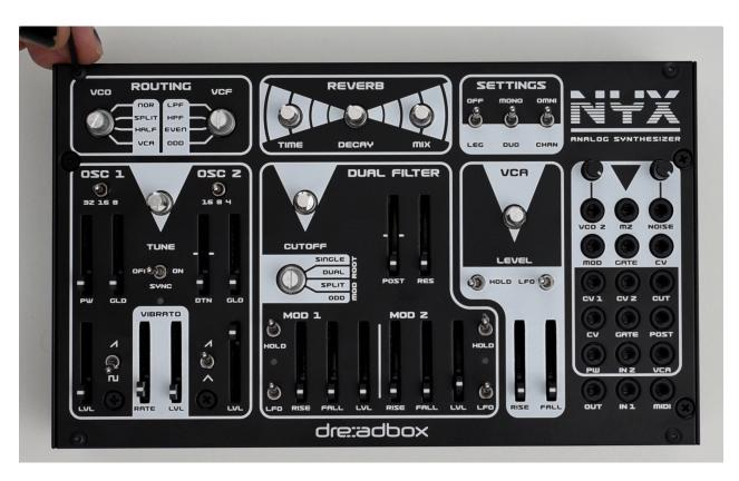
Screw in the pots and rotary switches, taking care that the rotary switches should not be overtightened but not too loose. The M10 nuts are for the rotary switches and the M8 for the pots.
