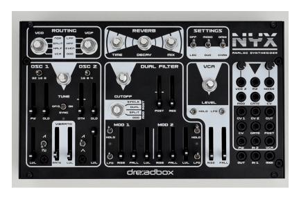
Screw the knobs to the pots and rotary switches as shown.
