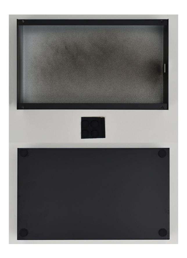
Place the unit in the metal enclosure. To easily achieve this, place the unit with the USB side first, and then push down the rest.
