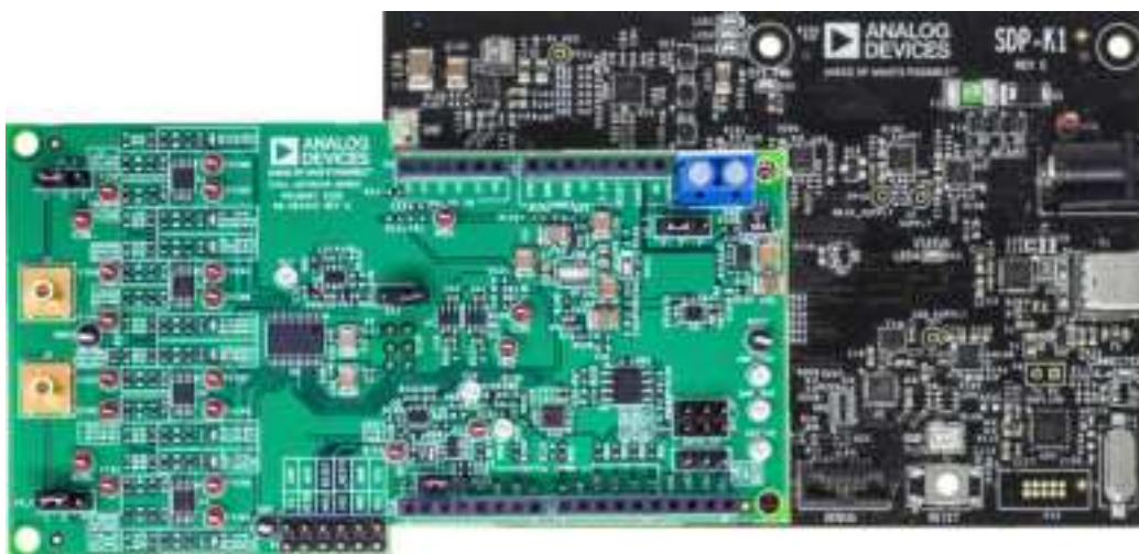
Figure 2. EVAL-AD7091R-8ARDZ (Left) Connected to the EVAL-SDP-CK1Z Board (Right)
