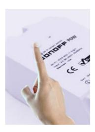
2. Press the button for 7 seconds until the green LED blinks like this: blinks 3 times and on repeatedly:
