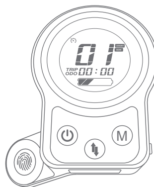
Figure 80: Push support controller buttons and components.
