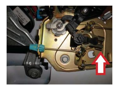
**STEP 2:** Attach the lift gate lock actuator into position.
