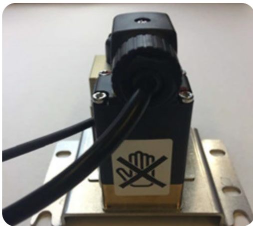
Magnetic valve for the measuring cell
