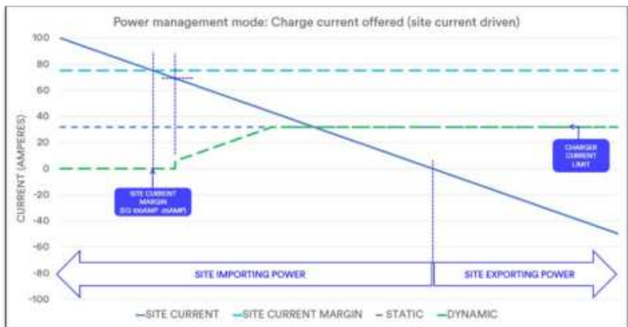
Figure 8: Power Management Mode: Charge current offered (site current driven) graph.
