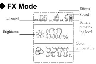
FX mode extends the functionality of the scene. If the controlled light does not have FX mode, adjust the SP and FX values and the light will not change.
