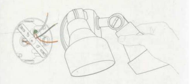
If there is a metal bracket attached to your junction box, remove that as well.
