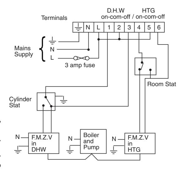
Other Danfoss Randall products suitable for use with above circuit:-AT cylinder thermostat; RMT room thermostat
