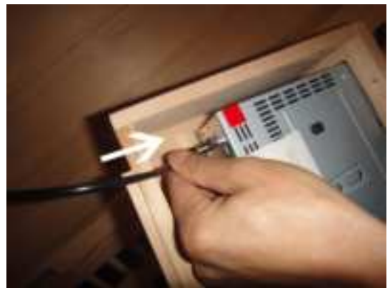
FIG-15.2 Connect antenna plug
