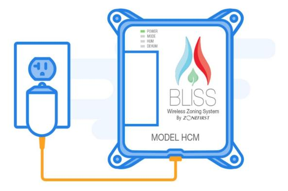
Power the HCM using the 12VDC power supply. The Power LED will turn on solid green.
