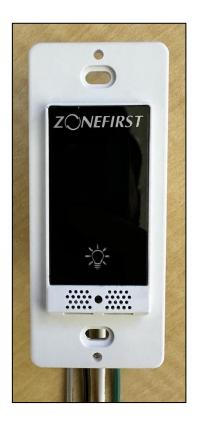
Located on the front of the LST is the touch display capable of interacting with the temperature input. Below it is an icon of a light bulb used to turn on and off the connected light source. At the bottom there are a variety of venting holes to read accurate temperature and humidity of the current room. At the center of the vent holes is a slightly larger hole which has a small tactile push button behind it. Using a small pin or a paperclip, you can push the button.
