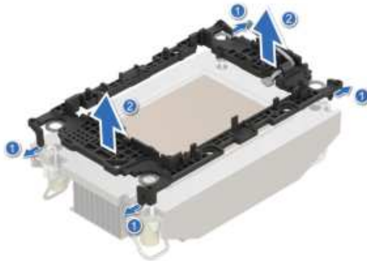
Figure 141. Removing the retaining clip
