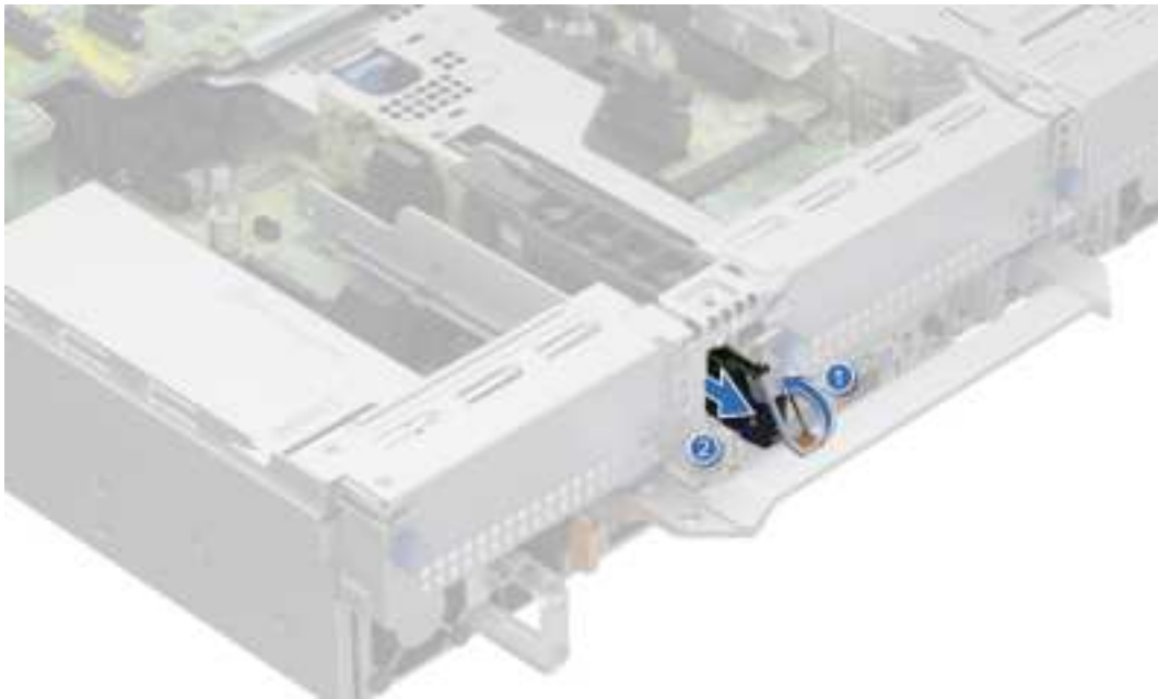
Figure 179. Removing the BOSS-N1 card carrier
