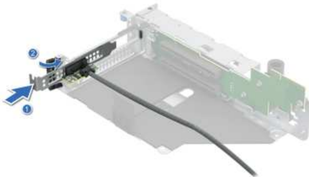
Figure 169. Installing the serial COM port
