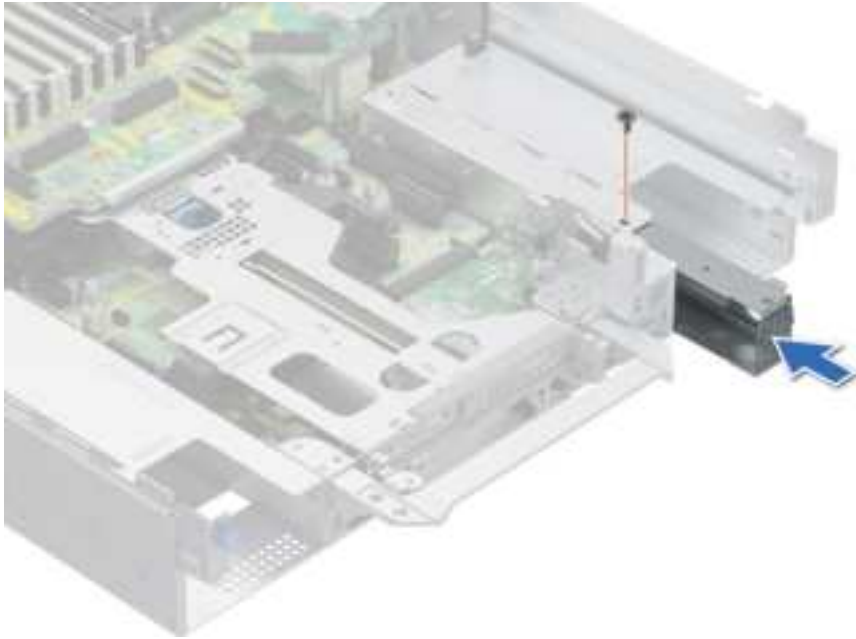
Figure 200. Installing a power supply unit adapter
