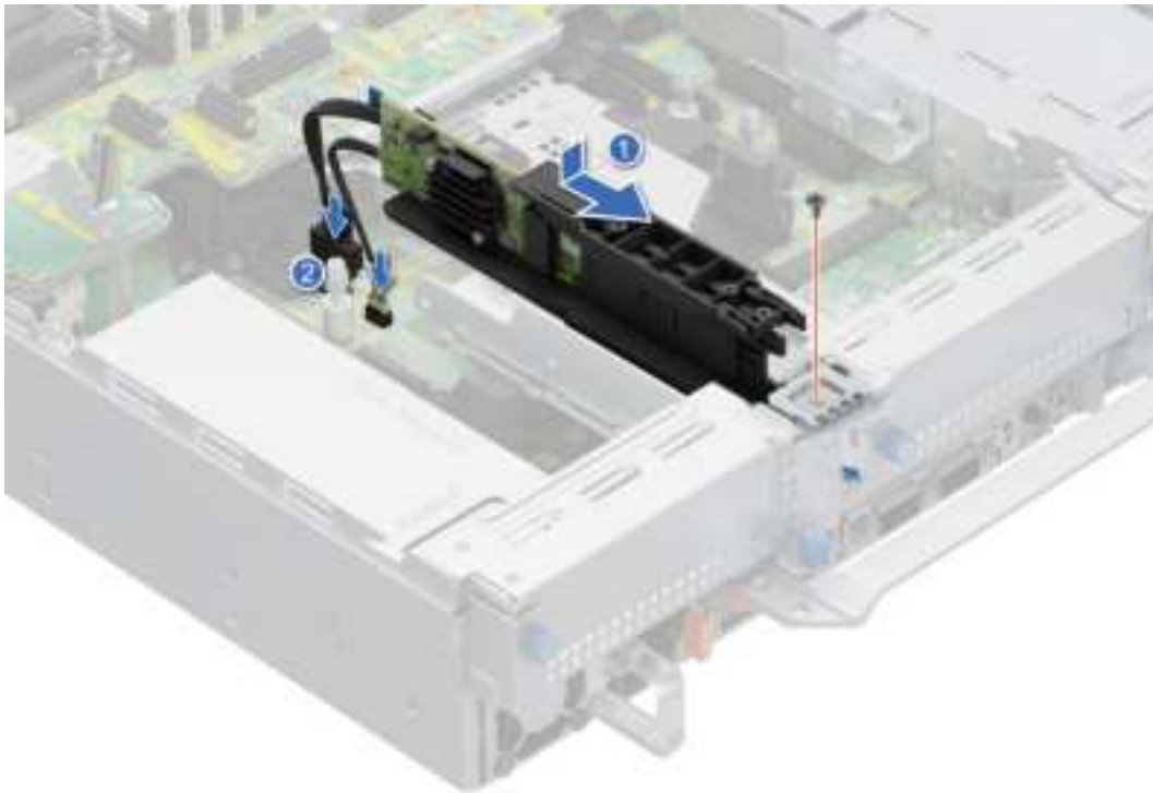
Figure 184. Installing the BOSS-N1 module
