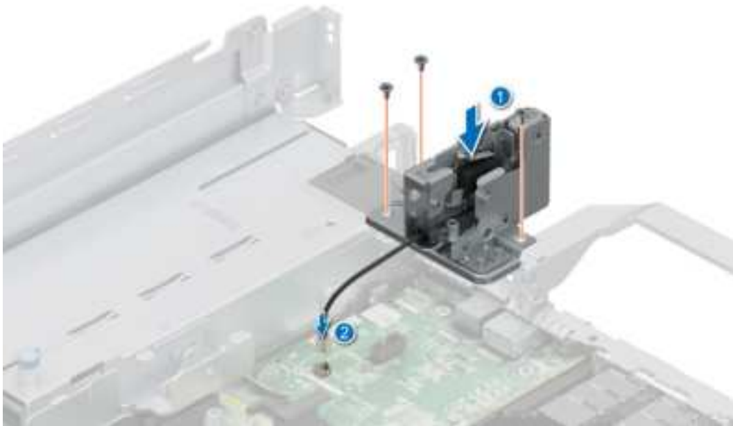
Figure 192. Installing the intrusion switch module
