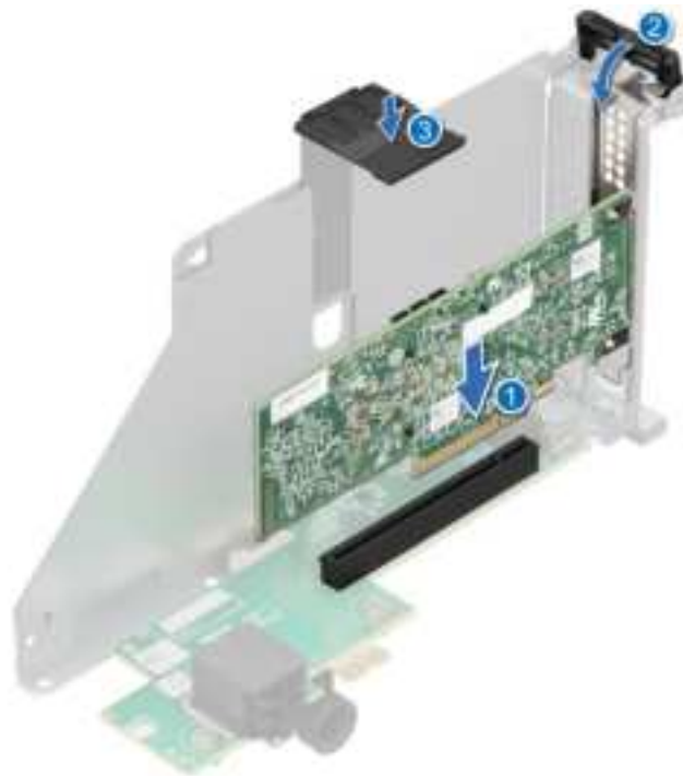
Figure 133. Installing an expansion card into the expansion card riser
