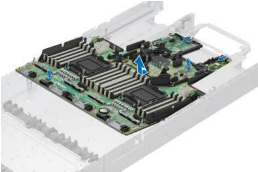
Figure 204. Removing the system board
