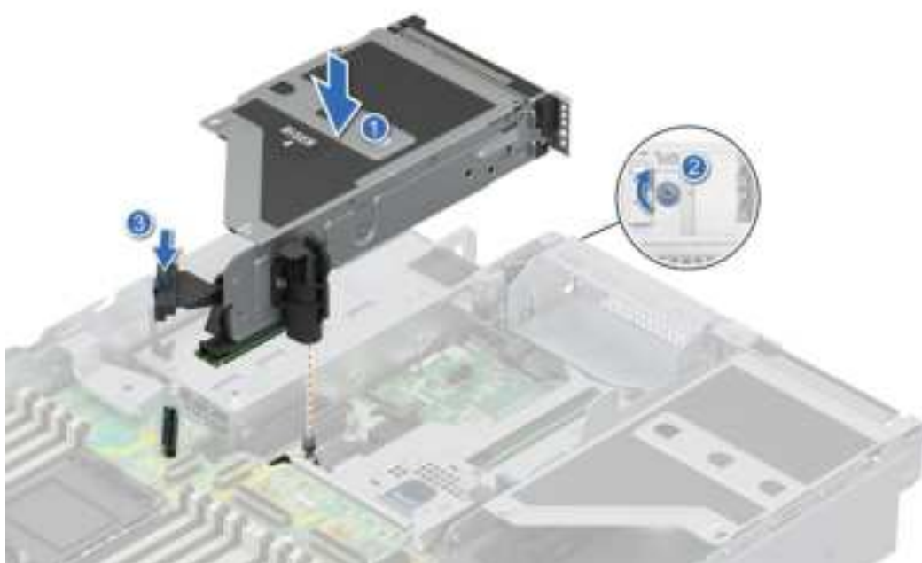
Figure 129. Installing the expansion card riser 4
