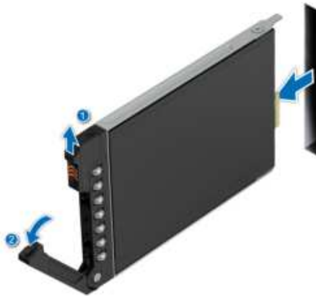
Figure 51. Removing an EDSFF E3.S drive carrier
