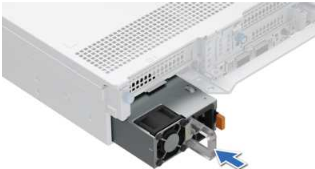
Figure 202. Installing a power supply unit
