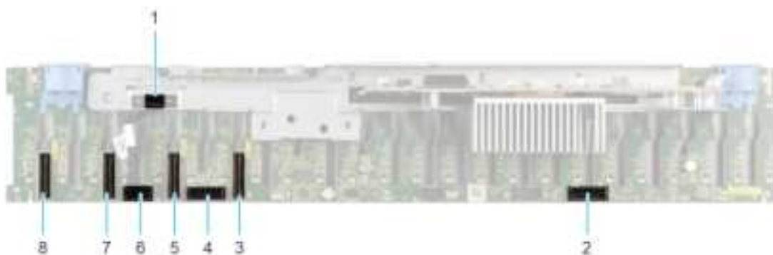
Figure 61. 24 x 2.5-inch drive backplane (front view)
