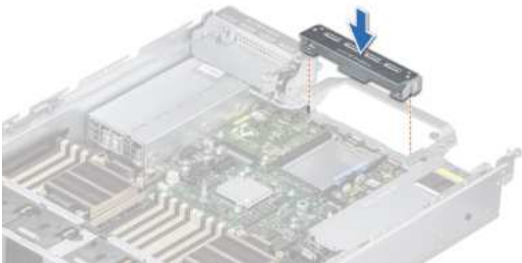
Figure 119. Installing the Riser 2 blank
