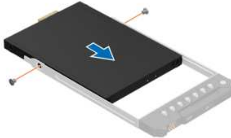
Figure 54. Installing the EDSFF E3.S drive into the drive carrier
