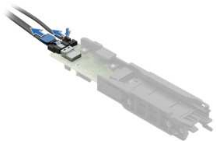
Figure 113. Removing the BOSS-N1 power cable and Signal cable
