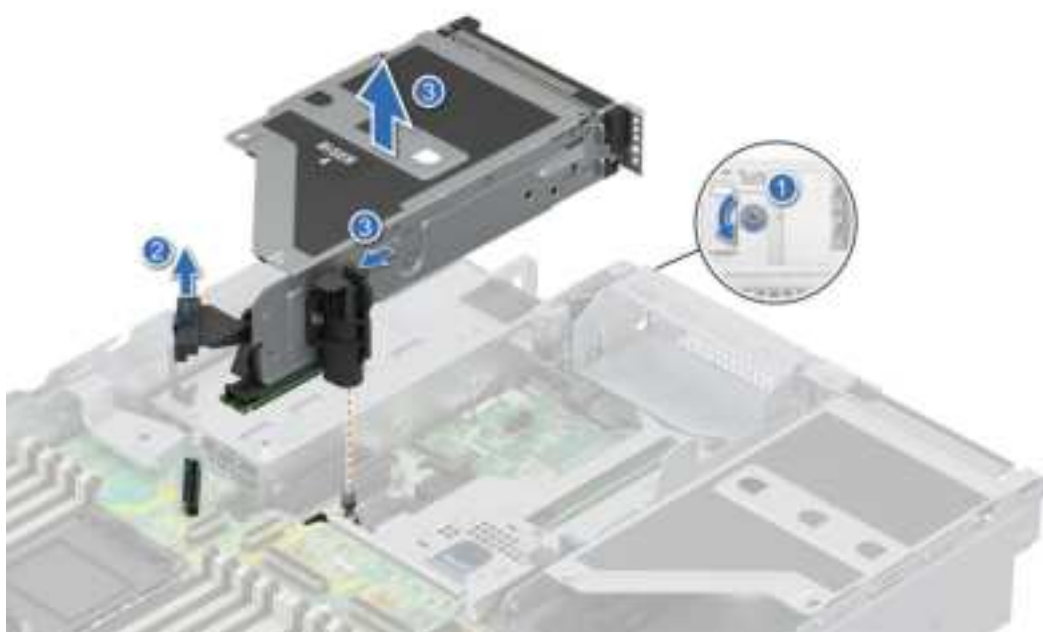
Figure 117. Removing the expansion card riser 4
