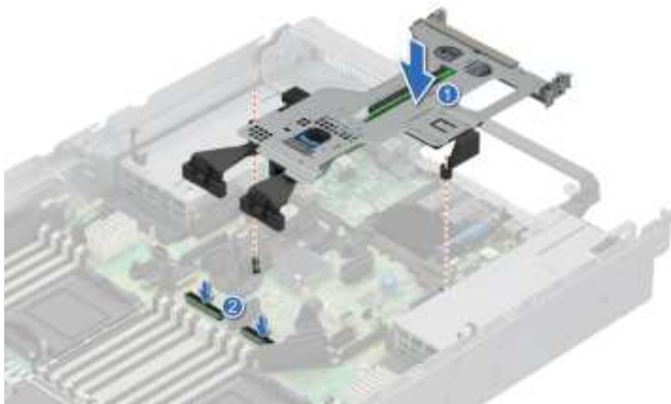
Figure 127. Installing the expansion card riser 2
