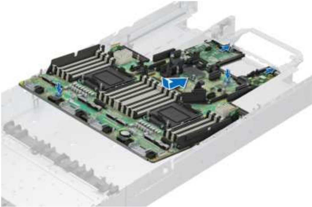
Figure 205. Installing the system board
