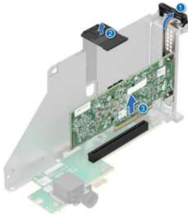
Figure 130. Removing expansion card from the expansion card riser
