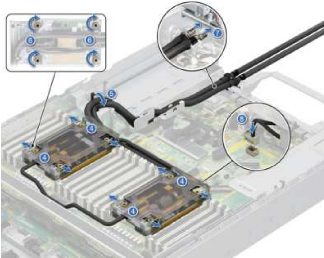
Figure 160. Installing the DLC module on PEM board
