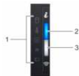
Figure 6. Left control panel with optional iDRAC Quick Sync 2 indicator
