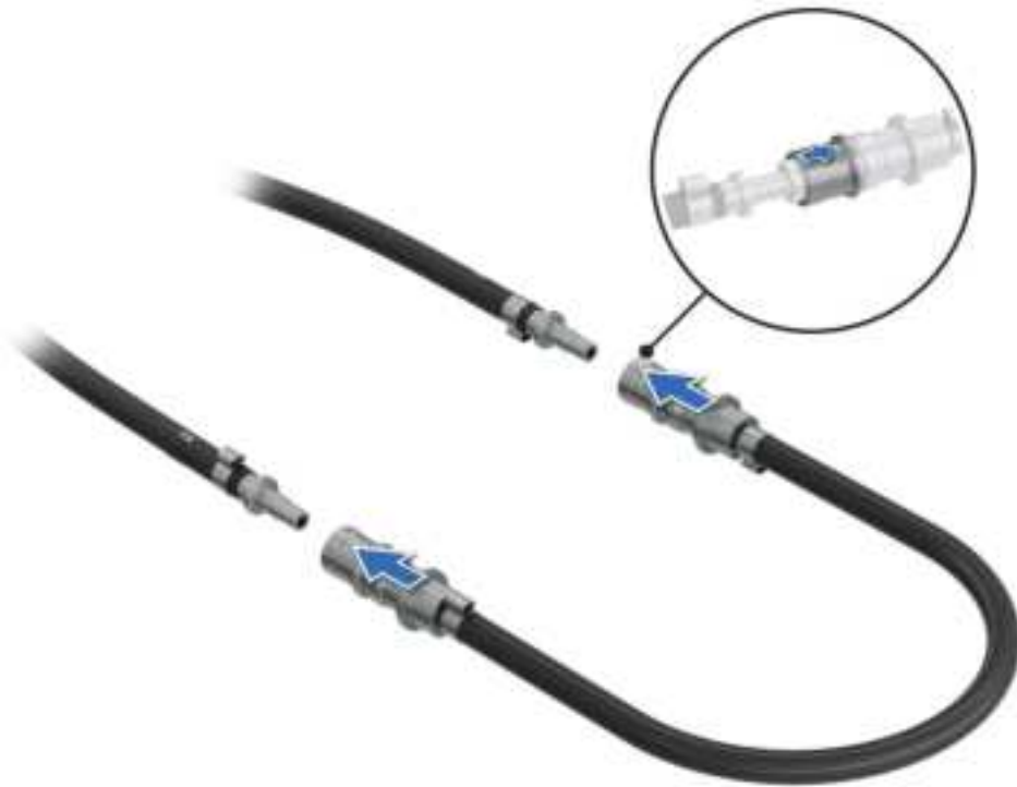
Figure 135. Installing the Freeze Expansion Loop
