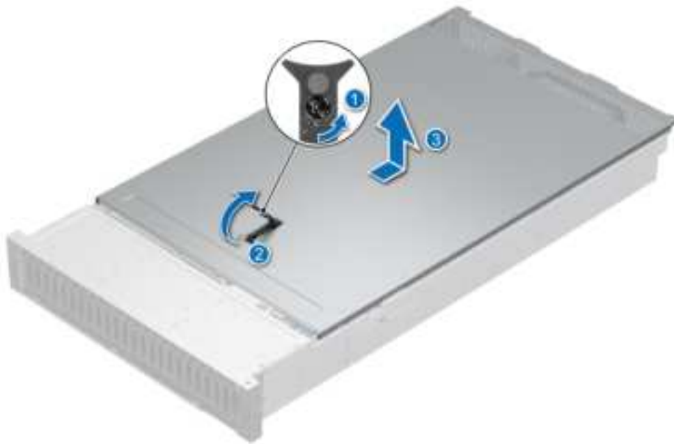
Figure 35. Removing the system cover
