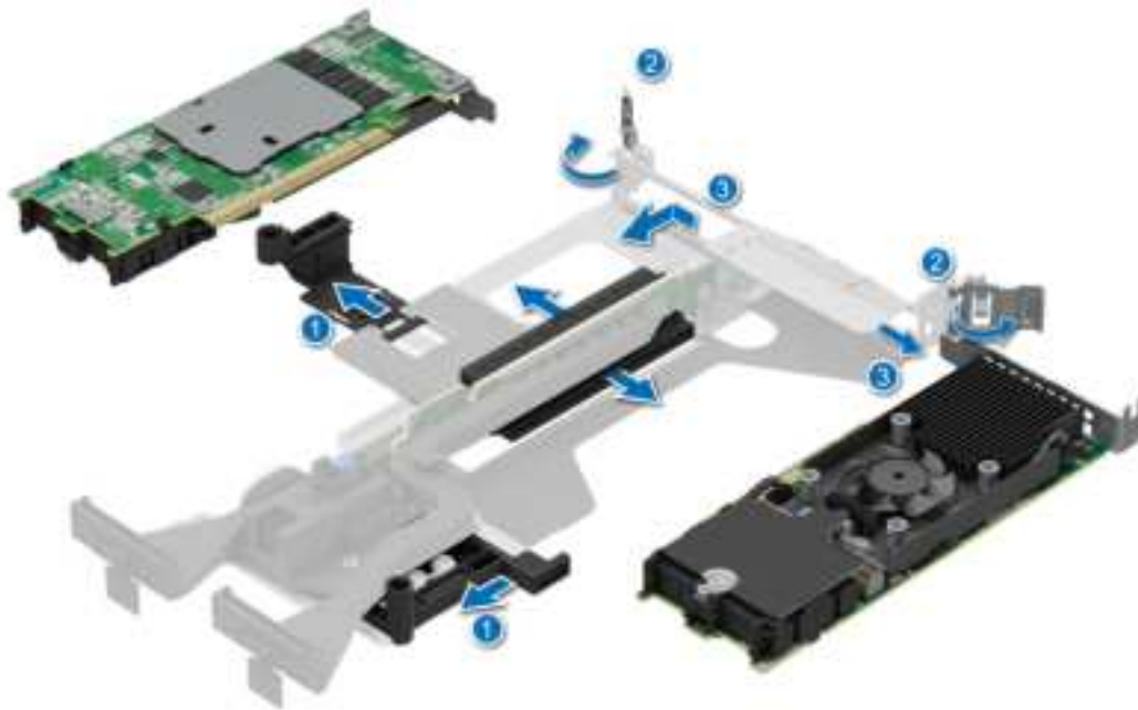
Figure 96. Removing the APERC module
