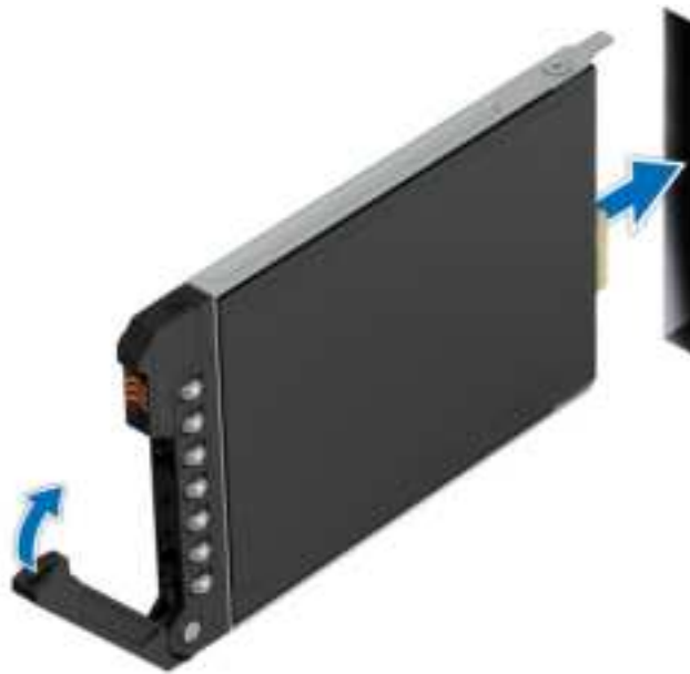
Figure 52. Installing an EDSFF E3.S drive carrier
