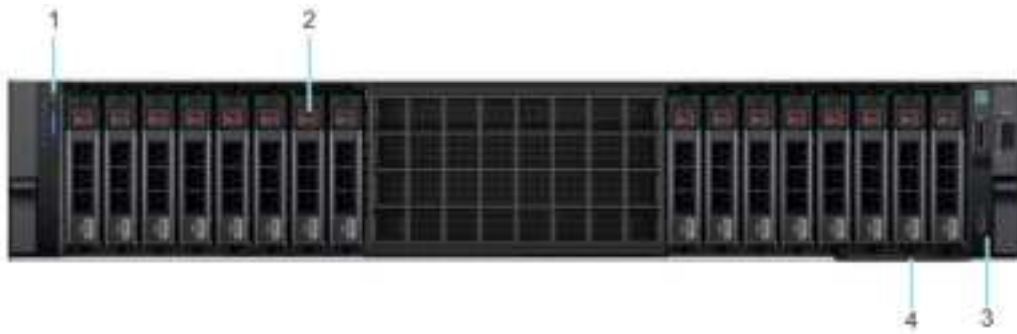
Figure 2. Front view of 16 x 2.5-inch drive system
