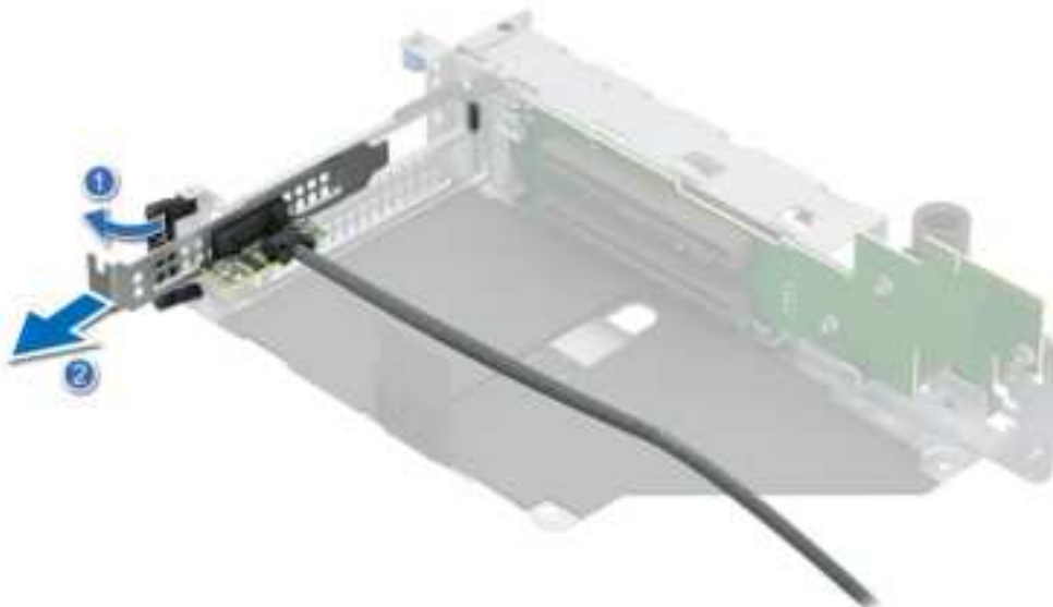
Figure 168. Removing the Serial COM port
