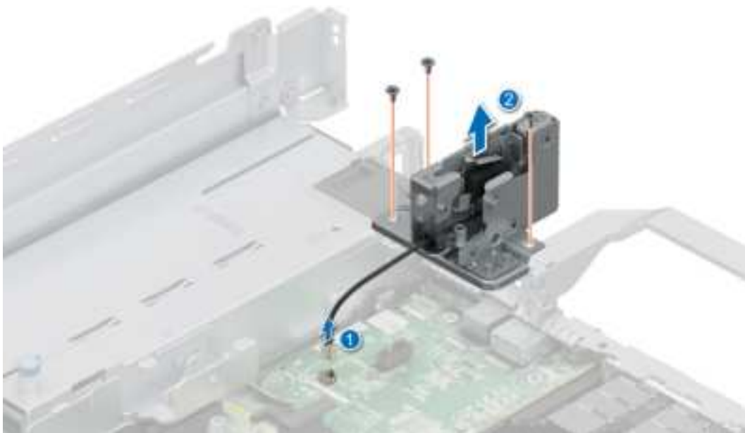
Figure 191. Removing the intrusion switch module
