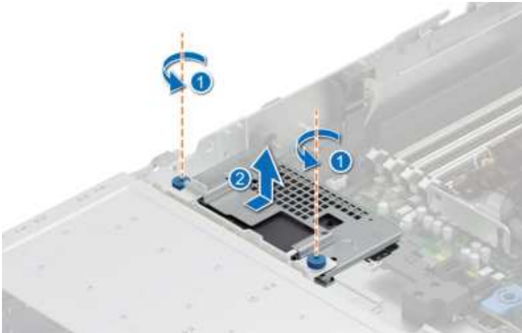
Figure 94. Removing the rear mounting front PERC module
