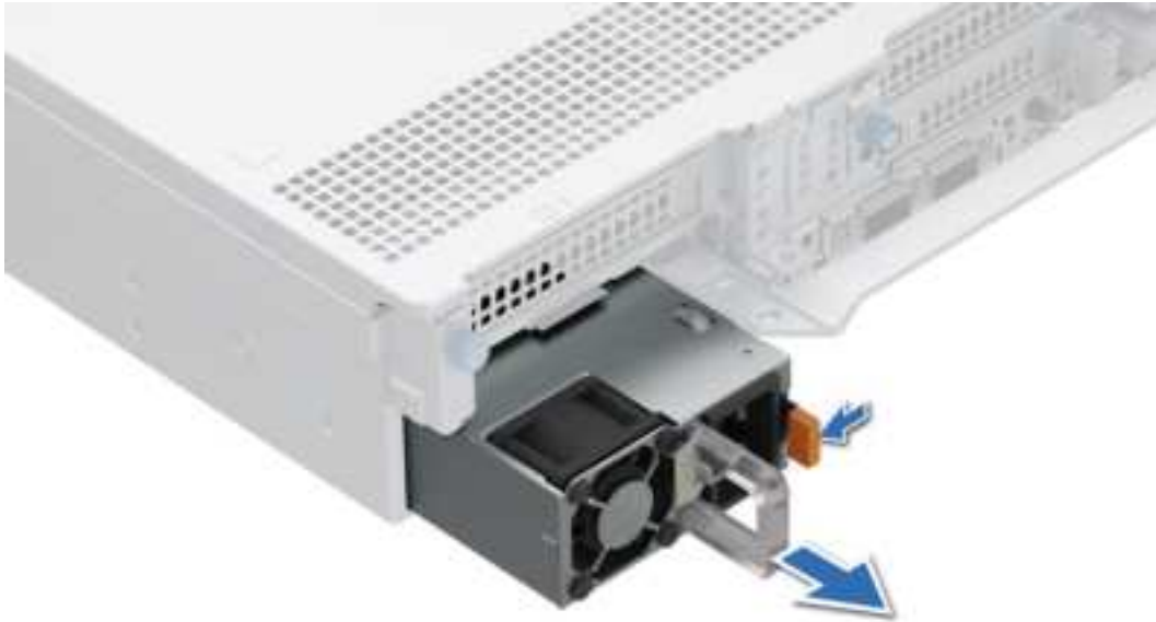
Figure 201. Removing a power supply unit
