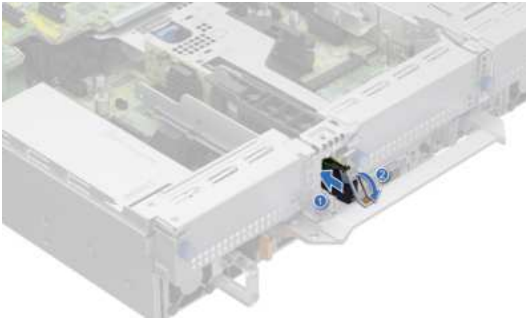
Figure 186. Installing the BOSS-N1 card carrier
