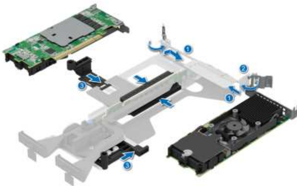
Figure 99. Installing the APERC module
