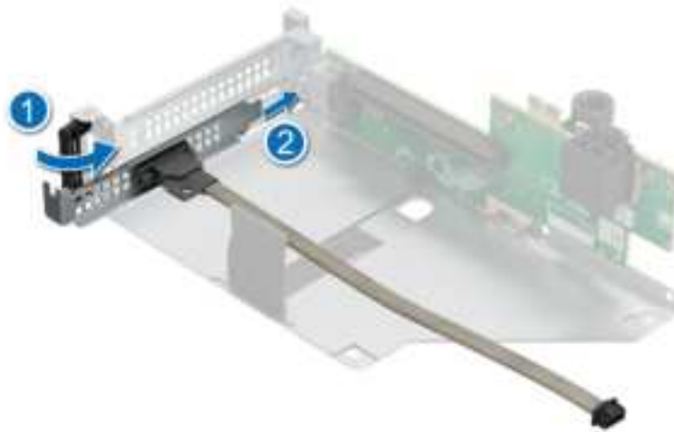
Figure 173. Installing the VGA port
