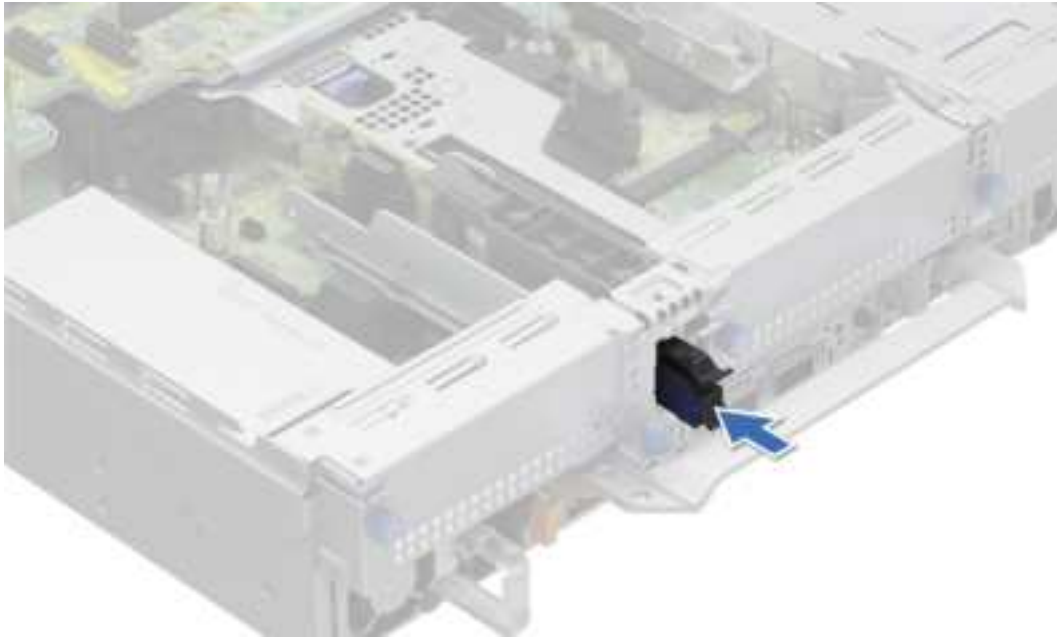
Figure 178. Installing the BOSS-N1 card carrier blank
