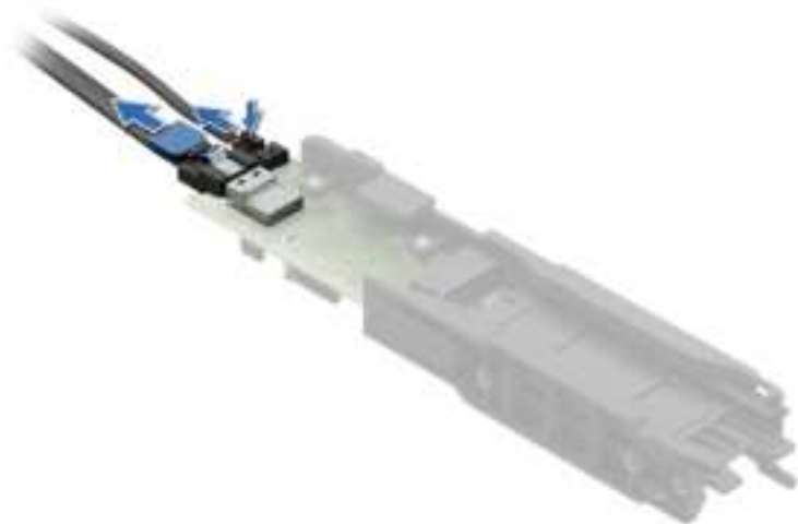
Figure 182. Removing the BOSS-N1 power and signal cable from the BOSS-N1 module
