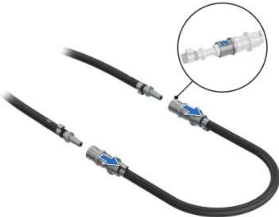
Figure 134. Removing the Freeze Expansion Loop
