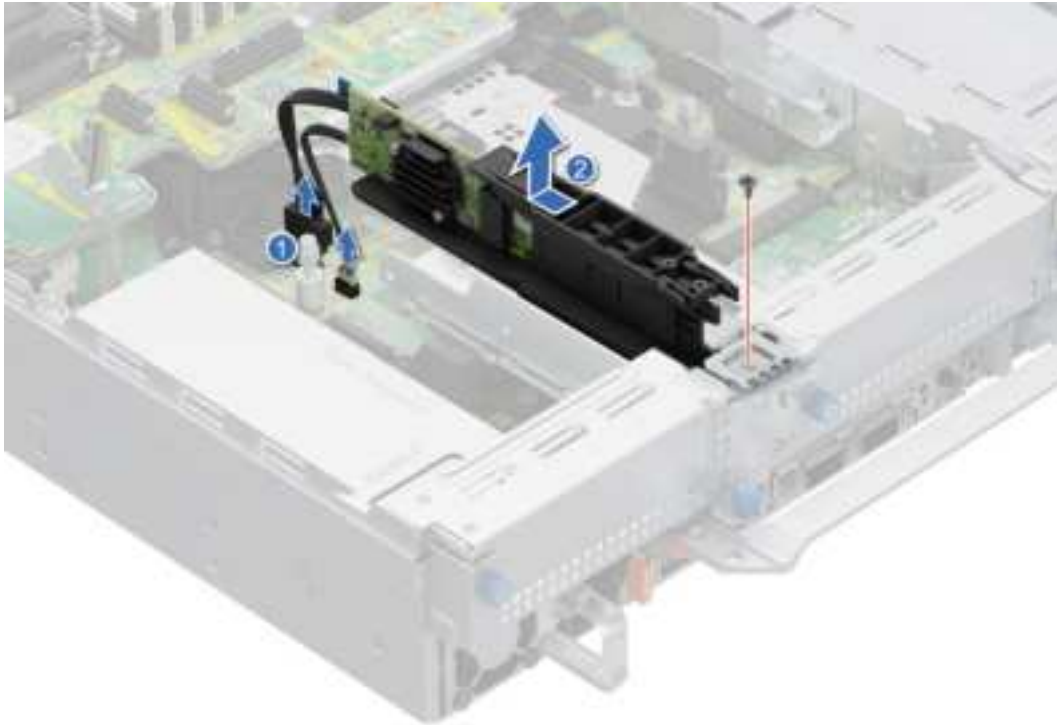
Figure 181. Removing the BOSS-N1 module
