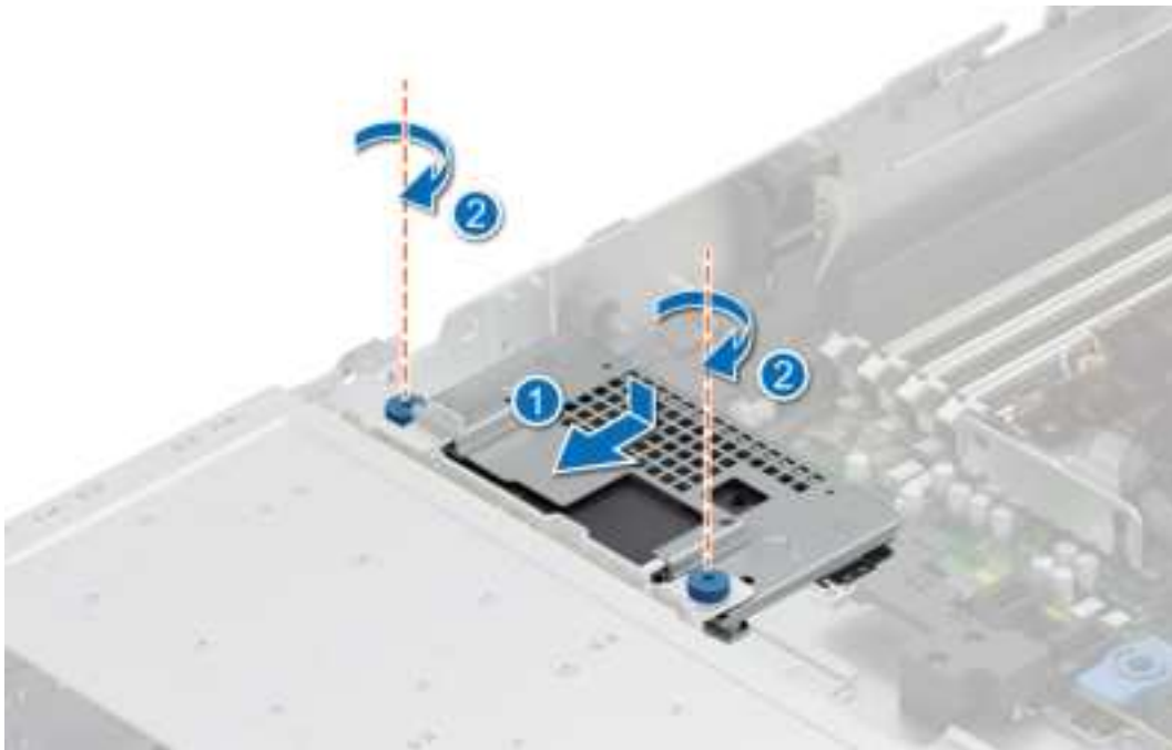
Figure 95. Installing the rear mounting front PERC module
