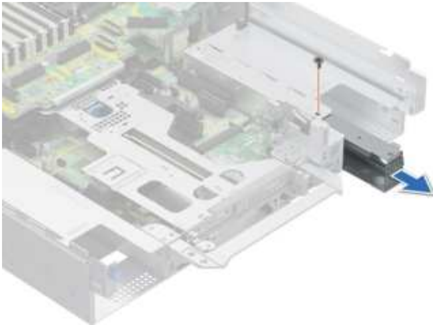
Figure 199. Removing a power supply unit adapter
