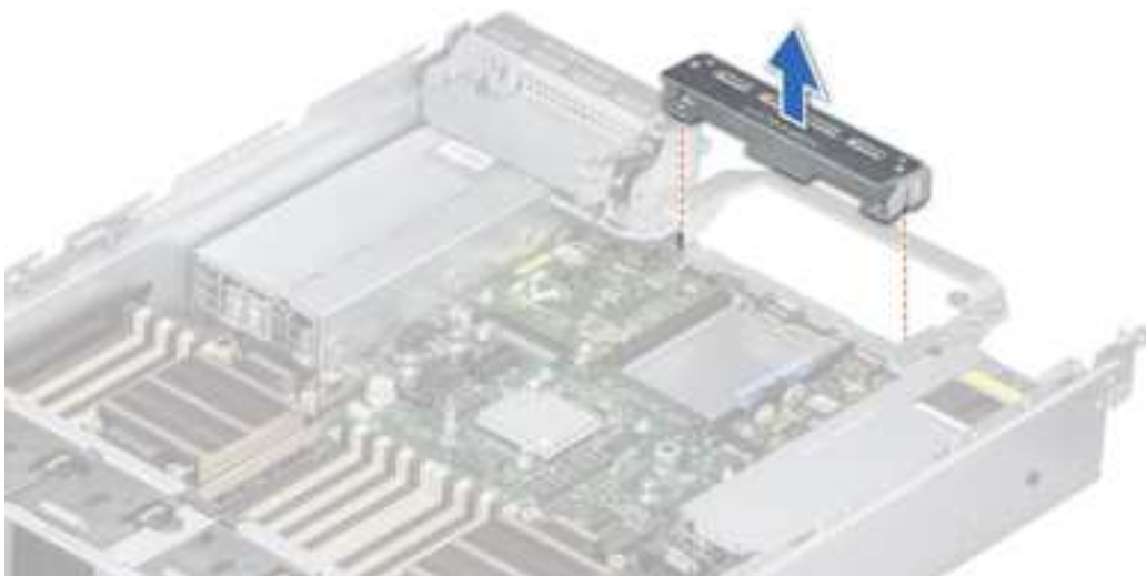
Figure 123. Removing the Riser 2 blank
