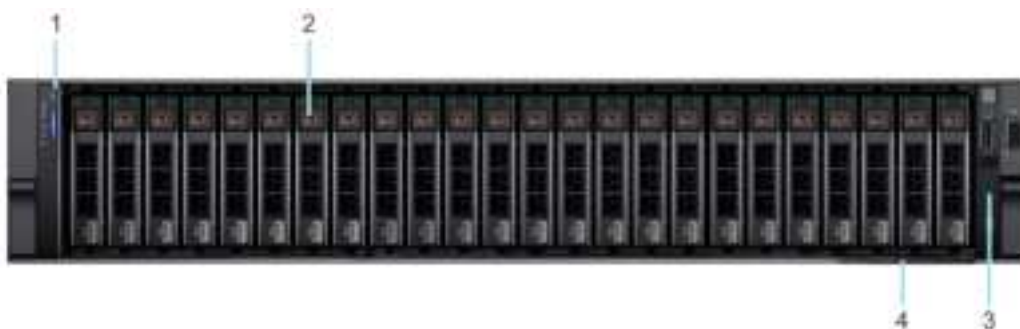
Figure 1. Front view of 24 x 2.5-inch drive system
