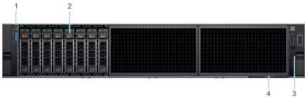
Figure 3. Front view of 8 x 2.5-inch drive system
