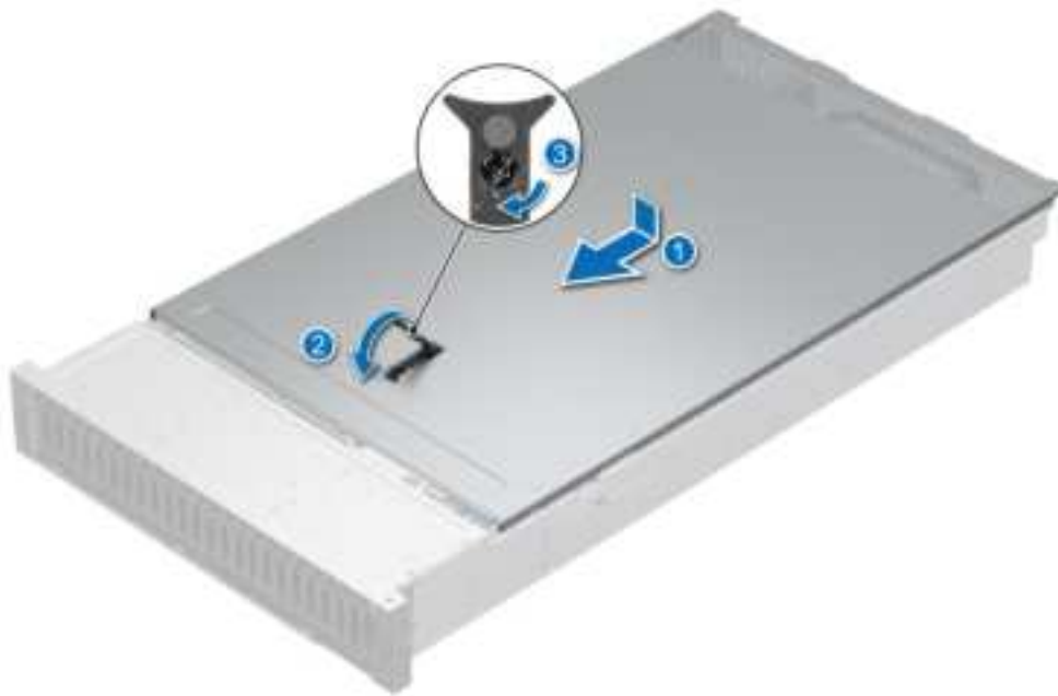
Figure 36. Installing the system cover
