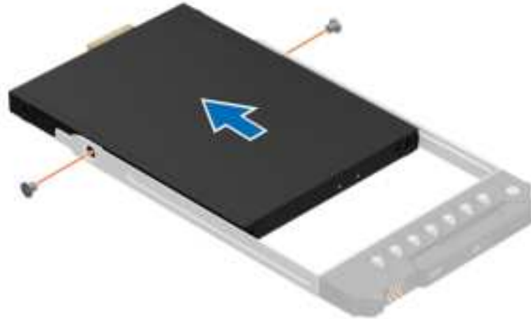
Figure 53. Removing the EDSFF E3.S drive from the drive carrier
