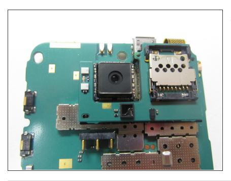
• The camera can be popped out easily using a blunt knife or credit card to pop it out. A new camera unit can be then simply put into the same place. In case a Nokia N900 camera unit cannot be found, it is possible to use a Nokia N79 camera without any ill effects.
