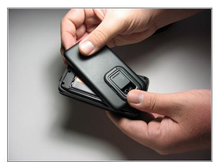
• In the case that you do need a new back cover remove it by locating the slit on the side of the phone allowing you to take off the cover, but if you need to further get to your camera you will need to remove the back cover as well.
