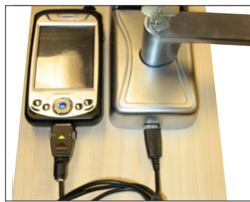
USB Connection with BM-150
