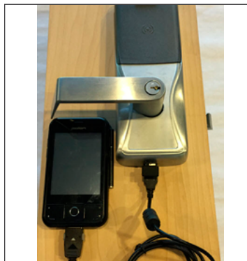
USB Connection with BM-170
