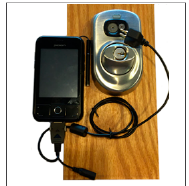
Serial Communication with 2PIN Serial Cable (BM-170)
