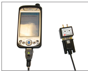
Serial Communication with CIP (BM-150 only)
