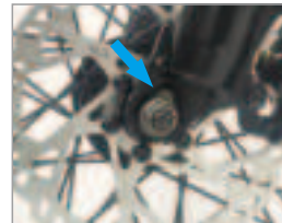
4. Tighten the left and right nuts as shown
