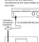
Note · Insert the plug of the calibration microphone all the way into the CALIBRATION MIC jack. If the calibration microphone is not connected securely, measurements may not be made properly.
