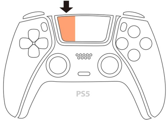
Press the left button while holding the TP Key
