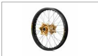
Tylne koło MXGP Replica (1,85" x 16") 5PA-F2075-9R-P0
