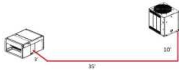
Figure 15. Allowable elevation difference: TTA or TWA below indoor unit
