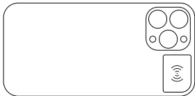
Figure 1 Common approximate location of the NFC chip on an iPhone
