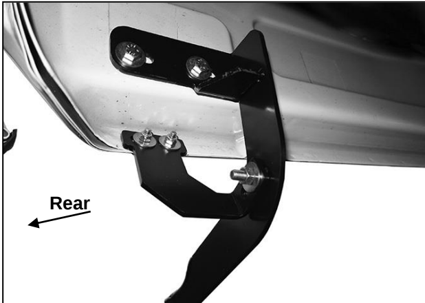
(Fig 16) Driver/Left rear Brackets installed
