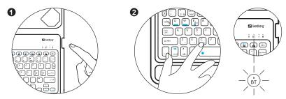
Keyboard ON Press FN +C, BT LED will flash ready to pair
