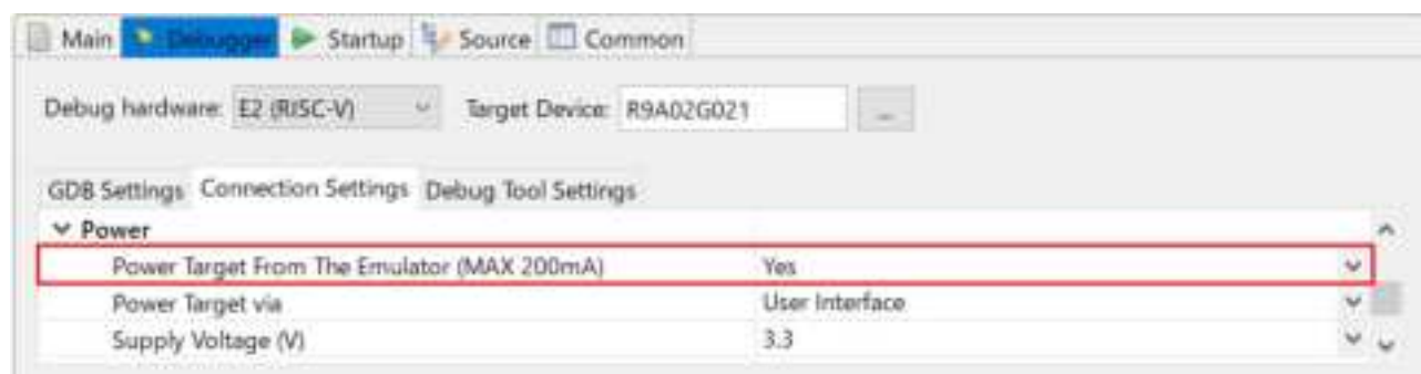
Figure 3-1 Setting for Supplying Power
