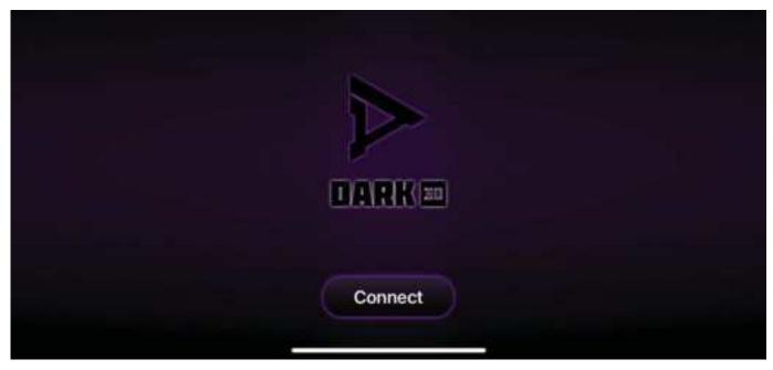
Press connect and the camera should connect to the app. If it does not connect, check to make sure you are still connected to the device's Wi-Fi. If you are connected to the device's Wi-Fi but are unable to manipulate your device, try closing and reopening the app.
