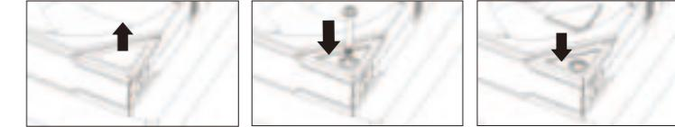
Secure the fan to the radiator and cover with the rubber pads to enhance
