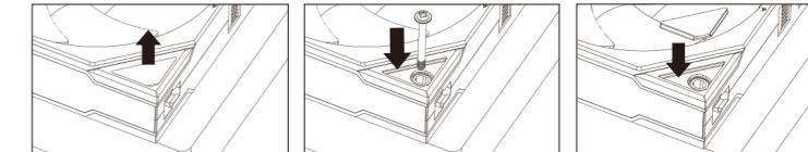
Secure the fan to the radiator and cover with the rubber pads to enhance the overall aesthetics/
