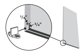
Install the hangers onto the door according to the measurement in the pictures below. Maximum door thickness is 13/4". If your door's thickness is less than 13/4", please add some bolt washers or cut the long door bolts to a suitable length to fit the door.
