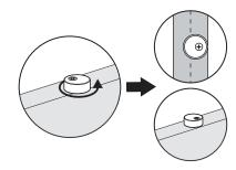
Adjust the 2 door stoppers to find a suitable position, Use the hex key to screw the door stoppers in place.
