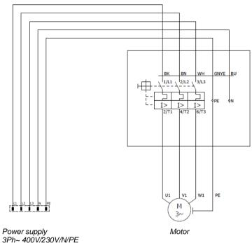
3Ph~ 400V/230V/N/PE 50Hz, max. 16/32A
